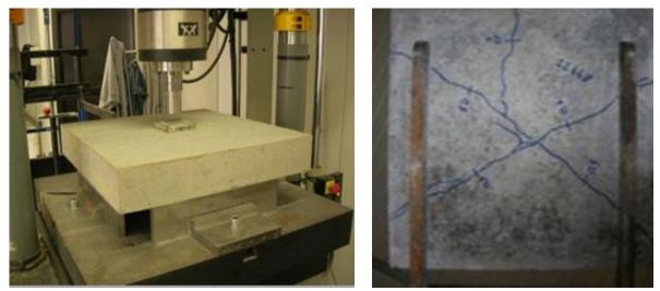
Figure 1 & 2: Square panel test according to EN 14488-5 (left) and crack pattern after 2 mm deflection (right)
