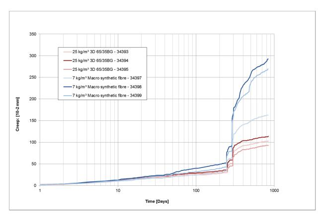
Figure 5: Creep behaviour of macro-synthetic and steel FRC
